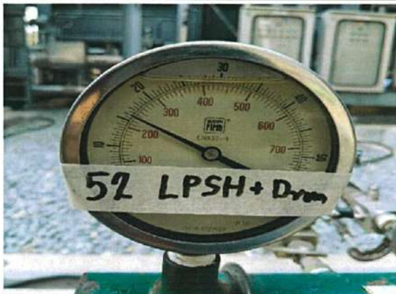
LP Loop Hydrostatic Pressure Test
