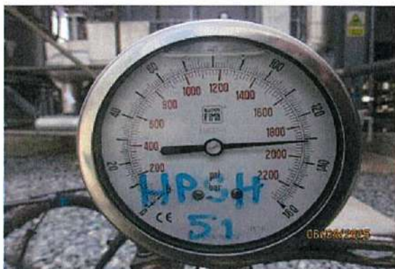
HP ECO Loop Hydrostatic Pressure Test 89.6 Bar
