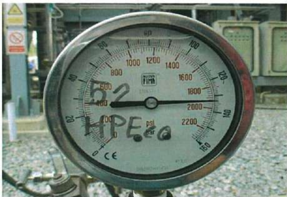
HP Loop Hydrostatic Pressure Test
