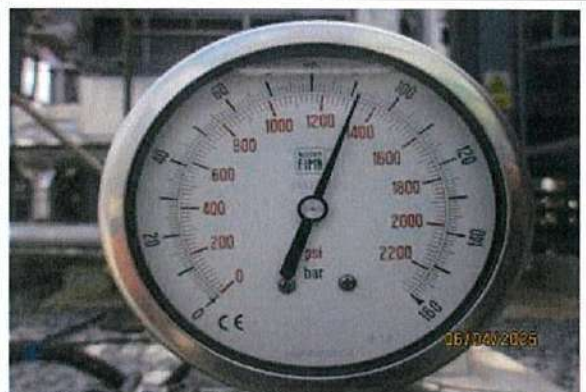
HP Drum + HPSH Loop Hydrostatic Pressure Test 89.6 Bar
